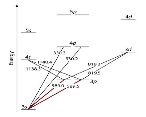
The fall of radiation with a wavelength of (589 nm) pushes the electrons from the 3s energy level to a number of excited sodium atoms to move to the 3p energy level as a result of absorbing the energy needed for their excitation. on the floating difference between 3s and 3p. In the case of sodium, the energy emitted by the return of the excited electron is in the form of a beam of a specific wavelength, which is the common yellow color of a sodium flame.
