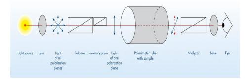
1-Radiation source, a sodium vapor lamp with a filter is often used to remove all unwanted streaks.
